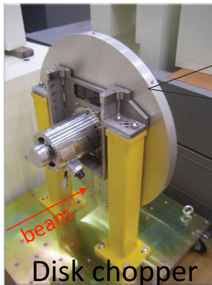
carbon-fiber-reinforced plastic (CFRP) containing B4C
